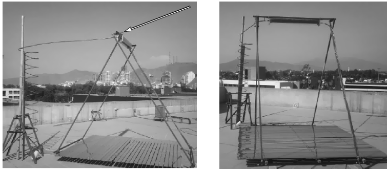
Fig. 8. Photographs of Fresnel linear distiller installed at University of Lima (Lima, Peru). White arrow indicates the heat absorber cavity in which boils seawater. Seawater inlet is on the right side of the cavity, steam outlet is on its left side and it is connected to a heat exchanger (tube in spiral shape).
