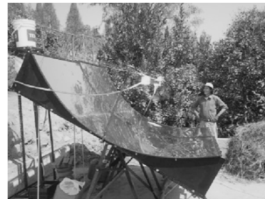
Fig. 4. Photograph of the PTC distiller installed in Cocayalta (Lima, Peru).
