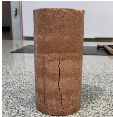
Figure 7: Cracks and fissures with mixture 2.
